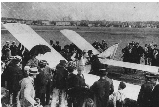
Figure 6. The Bleriot VI, a tractor monoplane with 'tandem' wings of nearly equal size fore and aft – after a hard landing (Bleriot 1907b).
