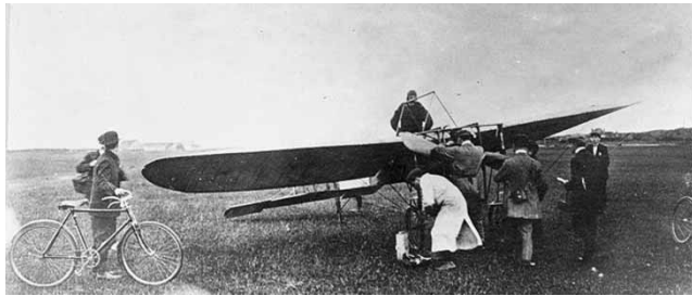
Figure 7. The Bleriot XI, a tractor monoplane with forward lifting wing, and rear rudder and elevator (Bain 2009).
