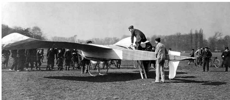
Figure 5. The Bleriot V, a pusher monoplane with forward elevator and rudder (Bleriot 1907a).
