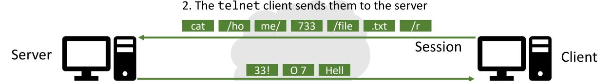
3. The TCP server stores data in its buffer Receive Buffer
