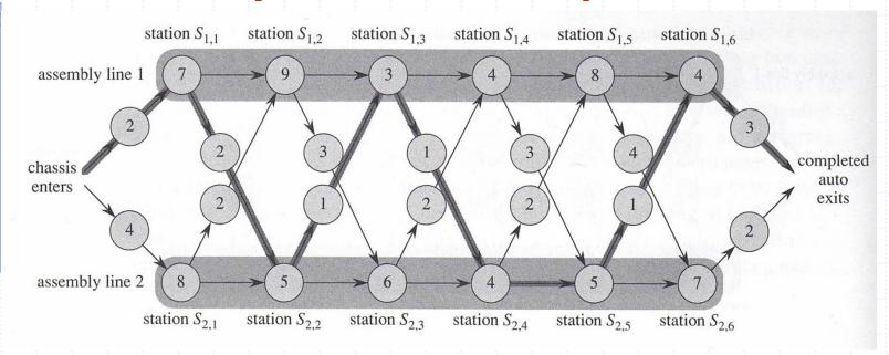
In this example, the fastest way through uses  $S_{1,1}$ ,  $S_{2,2}$ ,  $S_{1,3}$ ,  $S_{2,4}$ ,  $S_{2,5}$ , and  $S_{1,6}$
