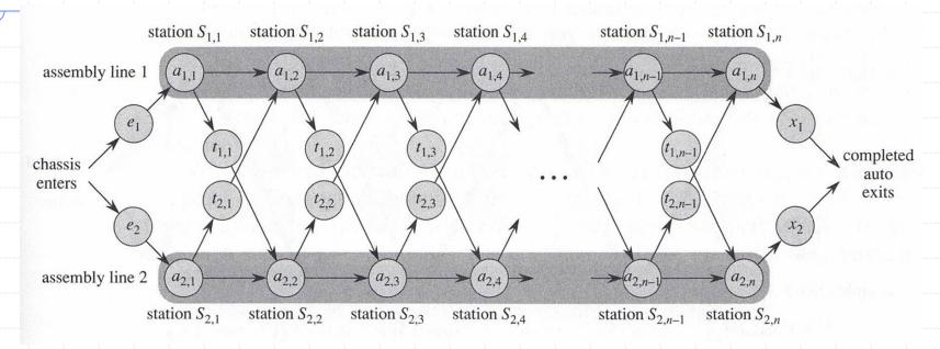
Two assembly lines, with processing and transfer times. Stations  $S_{1,j}$  and  $S_{2,j}$  do the same job.
