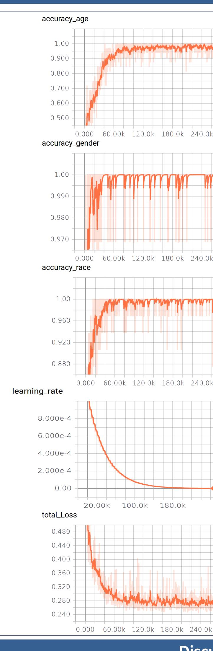
Figures on the left present the training results for the case of ARG prediction using a binning method and 9 classes for age. The figures on the right, show the case of considering 63 age classes. The network trained on 9 classes shows a much better performance in training and evaluation. This results show one of the disadvantages of conventional multi-task learning methods. Larger variations in the number of classes for each task will deteriorate the performance in multitask model.
