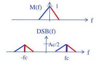
□ In SSB modulation, only one of the sideband (USB or LSB) is transmitted.
