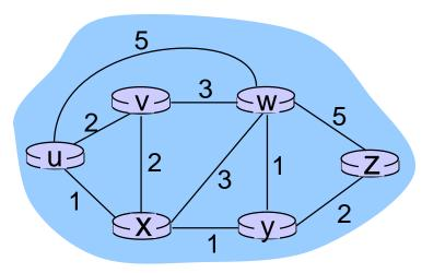
clearly,  $d_{v}(z) = 5$ ,  $d_{x}(z) = 3$ ,  $d_{w}(z) = 3$ B-F equation says:  $d_{ii}(z) = \min \{ c(u,v) + d_{ii}(z), i \}$  $c(u,x) + d_x(z),$  $C(u,w) + d_w(z)$  $= \min \{2 + 5,$ 1 + 3, 5 + 3 = 4 node achieving minimum is next
