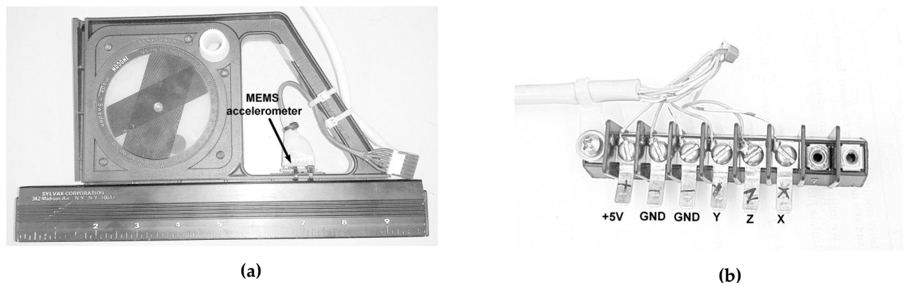
Figure 3: Inclinometer with mounted MEMS accelerometer (a); and MEMS accelerometer connections (b).
