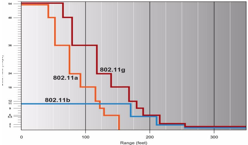
✓ As distance from the access point increases, 802.11 products provide reduced data rates to maintain connectivity.
