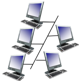
shared wire (e.g., cabled Ethernet)
